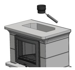
8. Install the first element, no. 5. Centre it on element, no. 4.
