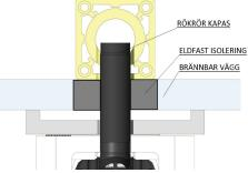
12. Install elements no. 7B, 8B and 9B in mortar. Secure the connection sleeve with insulation in the hole on the front. Let the connection sleeve protrude an equal distance to the thickness of the rendering (approx. 10 mm)
