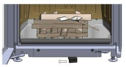
3. Let the first fire burn down with maximum air supply. This is to allow the stove to reach its operating temperature quickly. Light a new fire of the desired size and close the door. Wait a couple of minutes, until the fire has started burning properly. Then turn the damper to the left, until you have achieved a calm and harmonious fire.
