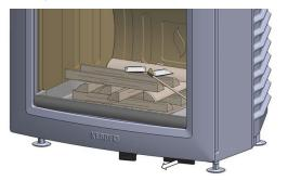
2. Push the damper control as far to the right as it will go, place a couple of firelighters on top of the heap and light. In the majority of cases, you can close the hatch immediately after lighting.
